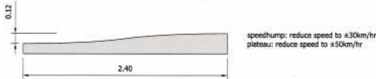
prefab concrete ramp with sinus-form RAMP TYPE A: sinus-form ramp
